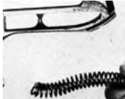
40. Disengage Mainspring and Mainspring Guide off the frame
