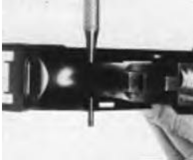
37. Push Recoil Lever Pin
